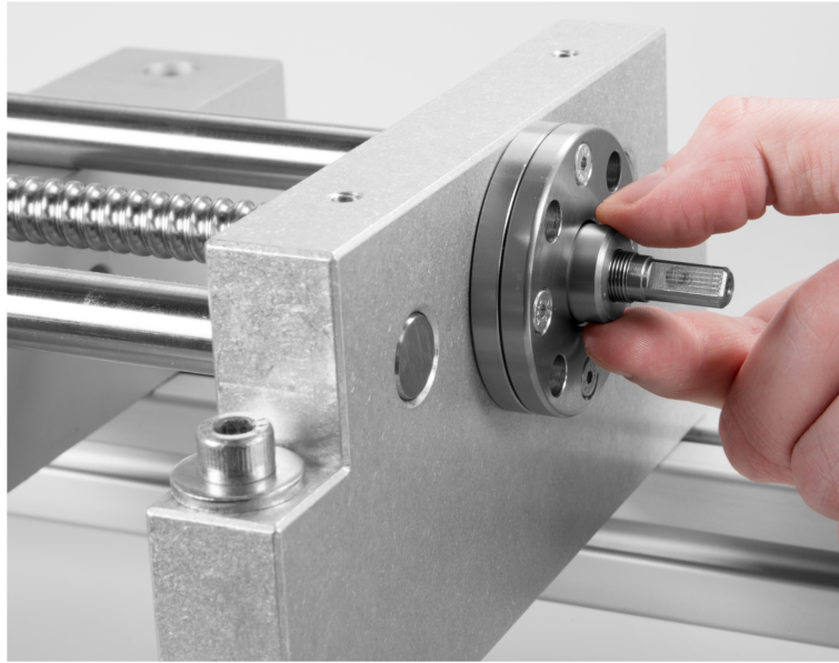
Figure 33. Removing the spacer from the center of the flange.
