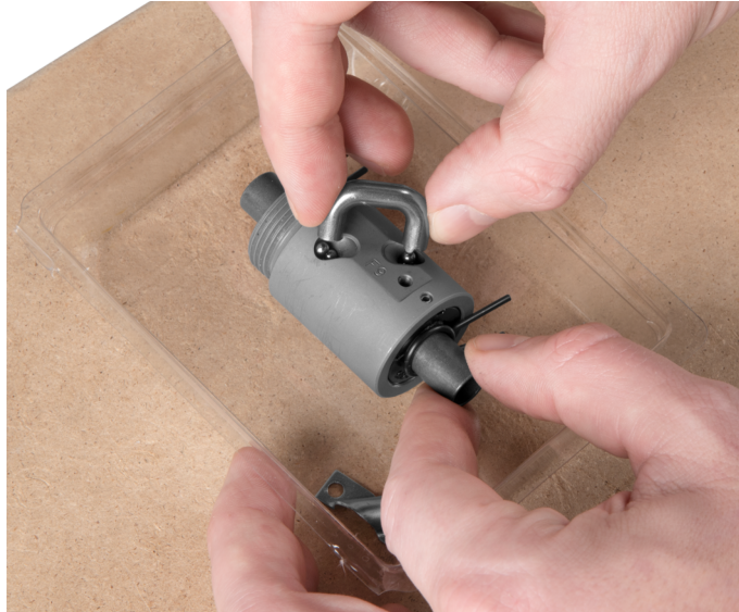
Figure 27. Removing the return pipe.
