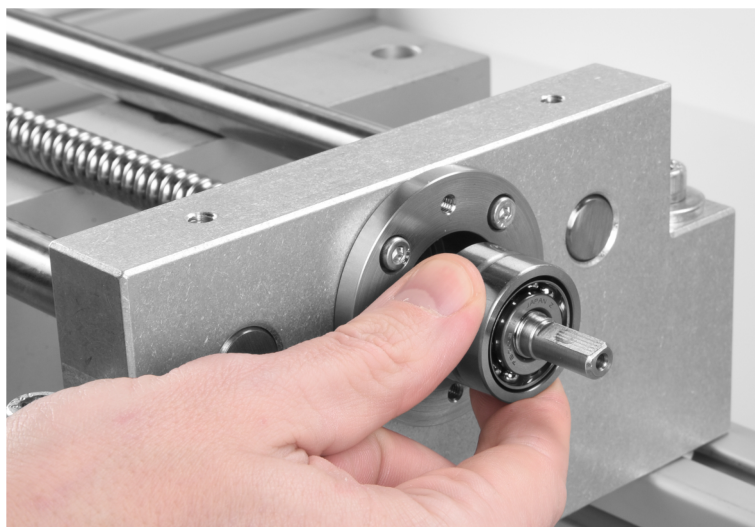
Figure 34. Removing the two angular contact bearings.
