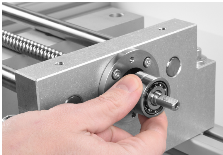
Figure 36. Inserting the angular contact ball bearings in the flange base.
