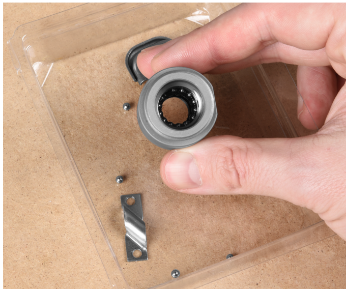
Figure 28. Removing the balls from the ball nut.
