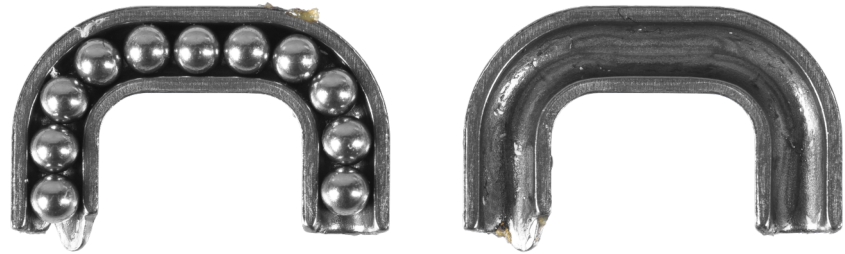
Figure 29. Filling one half of the return pipe with balls.
