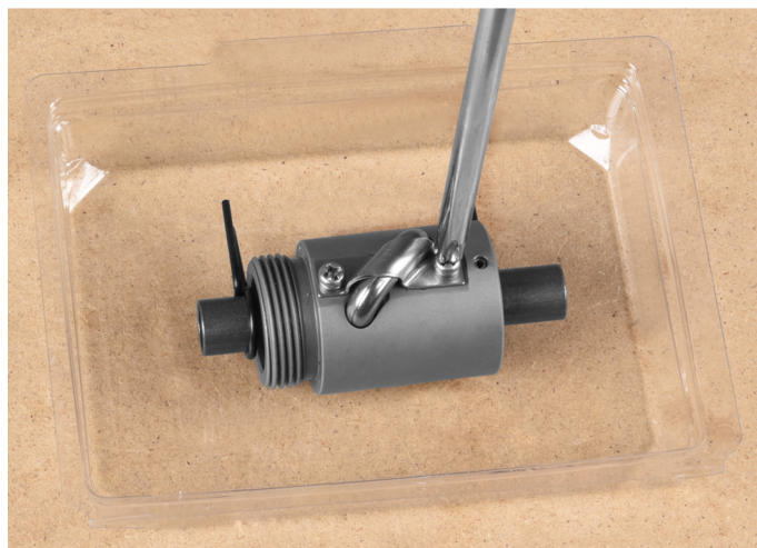
Figure 26. Unscrewing the screws of the return pipe holder on the ball nut.
