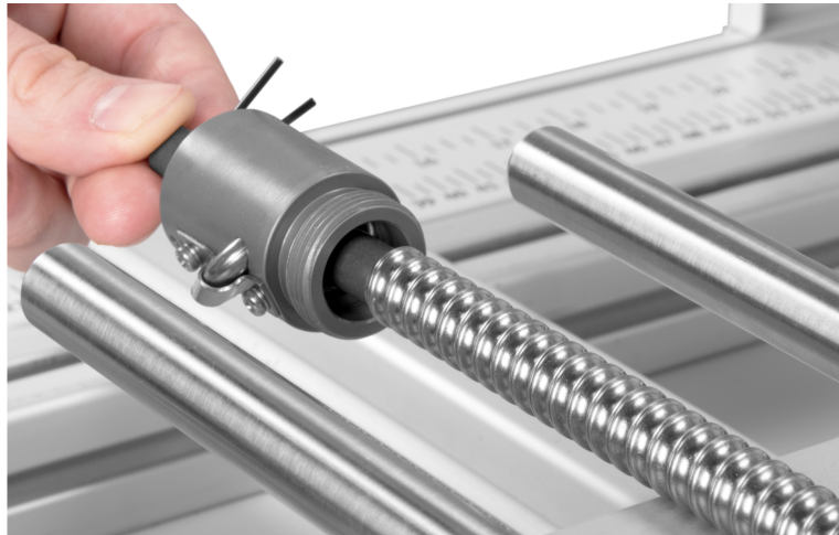
Figure 25. Sliding the ball nut on the arbor.
